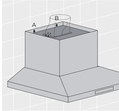
4. Fix exhaust transition duct using screws supplied (Fig. 8)
