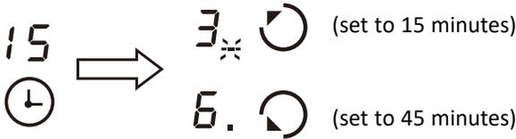
2. Once the set time expires, the corresponding zone will switch off. Then it will show the remaining time for the other heating zone and the dot for that zone will blink.
